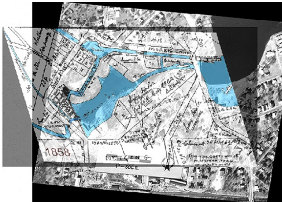
Figure 17. 1858 “Map of Lands Lying in Stanhope, New Jersey and Vicinity” .after being georeferenced and overlaid to scale over modern orth photo of project area. Screen shot of variable transparency GIS image off of Web. (Image courtesy of Davis Associates, July 2002).
