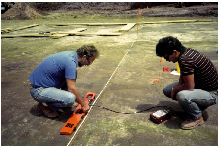
Figure 14. Mapping buried pit features with the EM-38 conductivity meter. Use of the instrument provided subsurface pit identifications without having to penetrate cultural features with electrodes.
