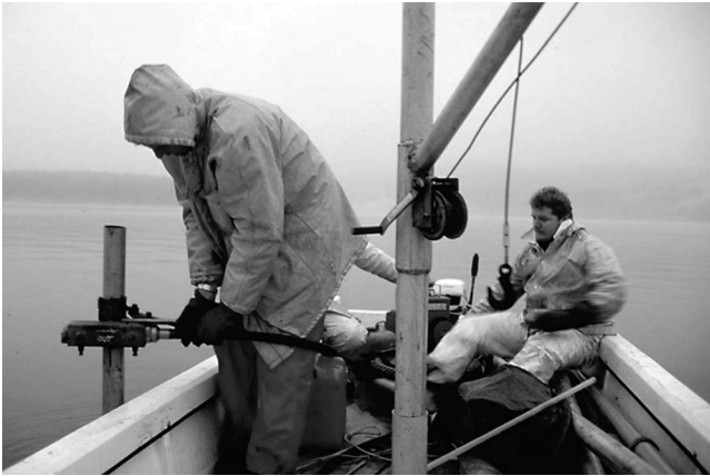
Figure 4. HASMAT team taking marine Vibracore sediment cores to define the Civil War-era Hudson River channel interface and historic sediment depths through trace element analysis in East and West Foundry Coves, Cold Spring, New York. Photo by Joel W. Grossman.
