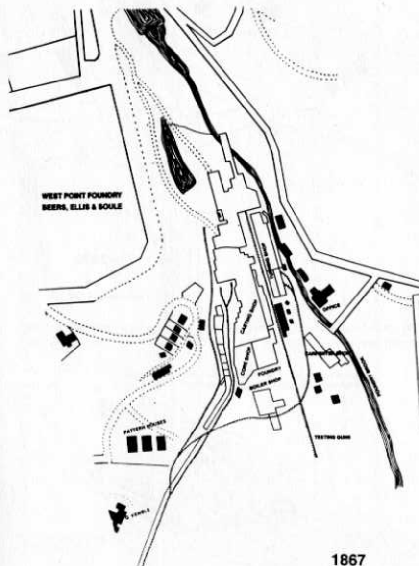
Fig. 11.5. Detail of 1867 Beers, Ellis, & Soule Map showing the "testing guns" rail line leading out of the gun casting and turning shops of the foundry and down to the shoreline area of the cannon-testing facility. Courtesy of Grossman and Associates, Inc.
